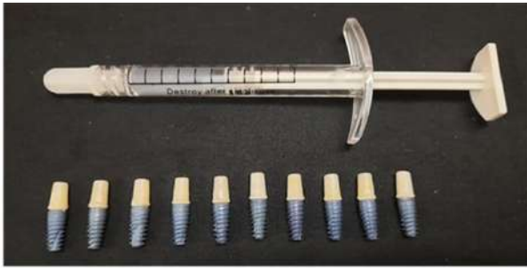
Fig. 5. Subgroup 2B-Zirconia abutments-Titanium implants-Sealant applied at IAI.
